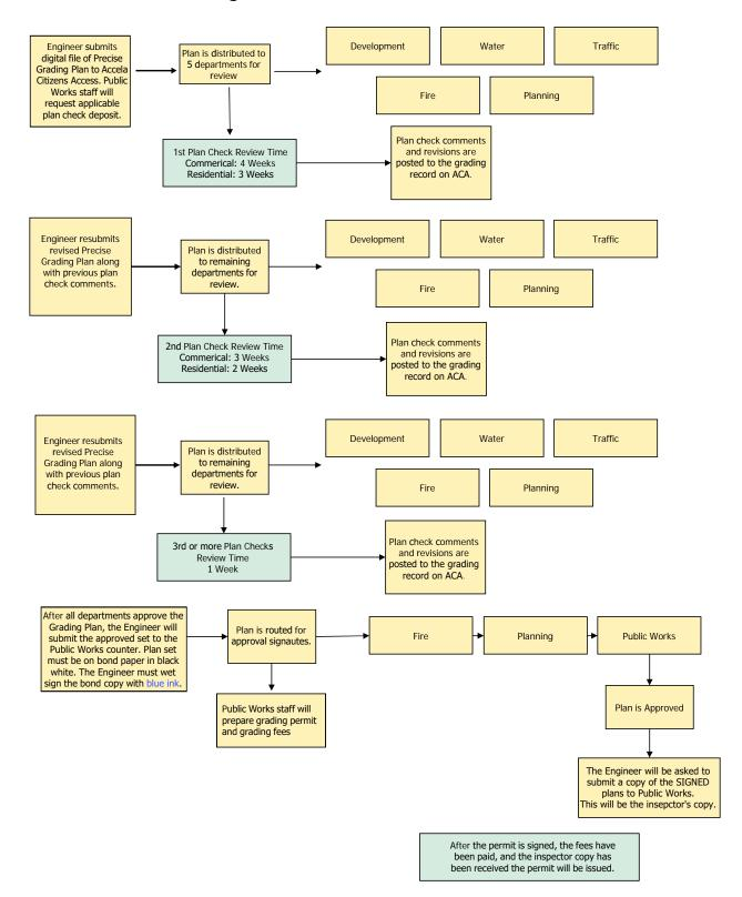
Note: The flowchart above demonstrates the typical process for a Precise Grading Plan. If the Code Requirements and/or Conditions of Approval for a project require the submittal of other reports/plans (i.e. Water Quality Management Plan, Hydrology & Hydraulics Study, Storm Water Pollution Prevention Plan, Easement Dedications, etc.), these items shall also be submitted to Public Works with the first plan check of the Precise Grading Plan.
