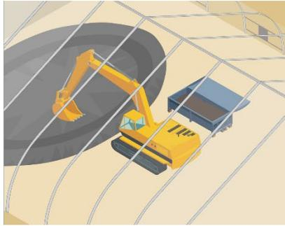
Excavated Pit F waste will be loaded into bins which will be sealed for transportation while inside the tent
