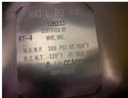
Figure 2. Example of a CO<sub>2</sub> Manufacture Plate
